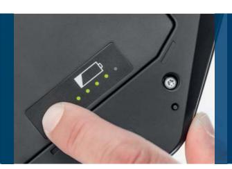
Smart battery management A fully charged battery lasts for up to 24 hours. The battery status is indicated by the LEDs on the battery pack.
