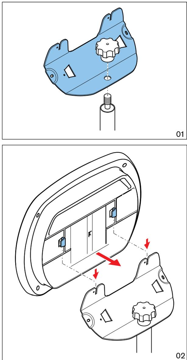
**Figure 5.4: Mounting on a tripod floor stand**
