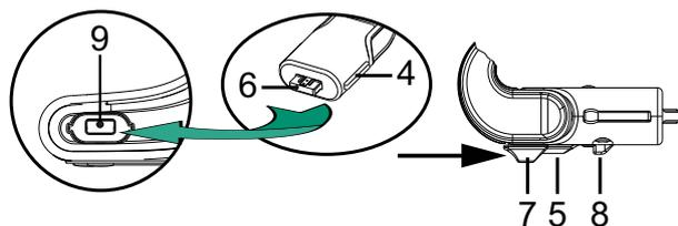
**Figure 6.3: DCNM-HDMIC or DCNM-MICS / DCNM-MICL connection**
