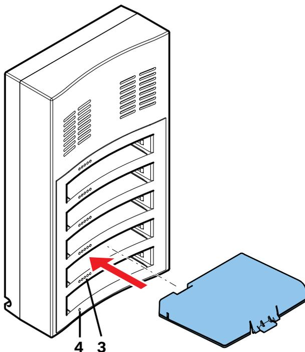
**Figure 6.8: Placing of the Battery Pack****Charging time**
